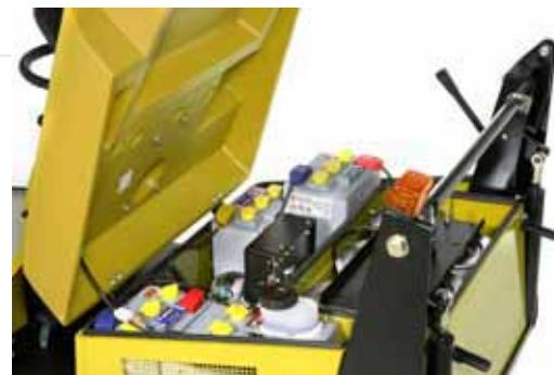
*option 4 batteries 6v-180ah (5h)*
